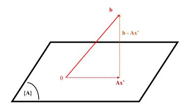
$x^*$  is the best approximation to b from the subspace span{A} iff (b - Ax) is  $\perp$  to the whole subspace span{A}. This in turn is equivalent to Normal equations  $A^{\top}(Ax^* - b) = 0.$
